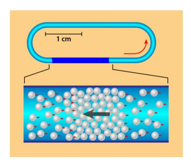
(Top) Sketch of the setup used by Bartolo and colleagues [1]. Millions of microbeads, which roll upon the application of an electric field, explore a centimeter-sized racetrack-shaped enclosure. (Bottom) The flock of particles with aligned velocities (red arrows) can be arrested by the formation of large
