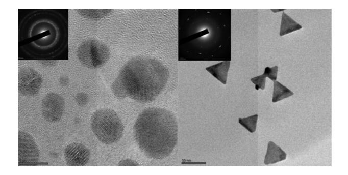
When gold is deposited on "dirty" graphene (left), blobs of gold collect around impurities. But when gold grows on graphene that has been heated and cleansed of impurities (right), it forms perfect triangles of gold. Credit: Kate Reidy/MIT
