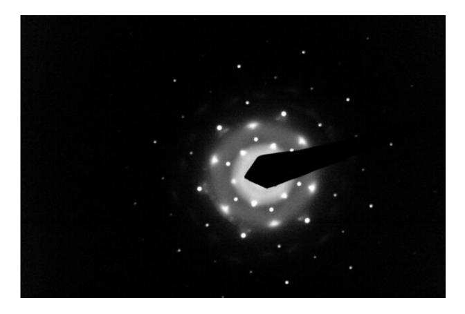
An electron diffraction image of niobium deposited on top of graphene shows that certain crystal planes of niobium align with the crystal planes of the graphene, which is known as epitaxial growth. When a 3-D material is grown on top of a 2-D layer, this perfectly aligned atomic arrangement is often important for device makers. Credit: Kate Reidy/MIT
