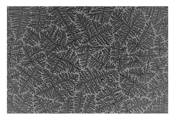
Niobium deposited on top of graphene produces structures that look like the frost patterns formed on the inside of windows in winter, or the feathery patterns of some ferns. They are called dendritic structures. Credit: Kate Reidy/MIT
