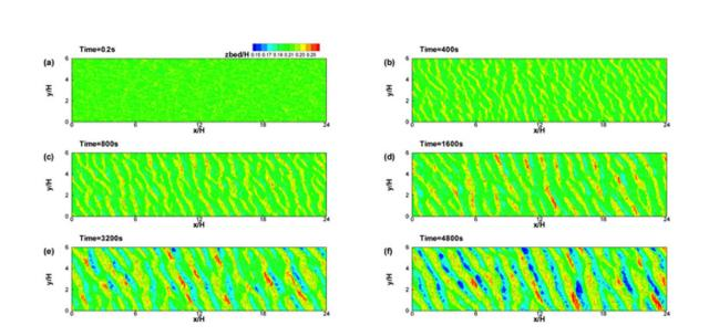
Simulated sand wave initiation in 3D contours of bed elevation corresponding to a) t=0.2 seconds, b) 400 seconds, c) 800 seconds, d) 1,600 seconds, e) 3,200 seconds, and f) 4,800 seconds. Credit: Hongwei Fang
