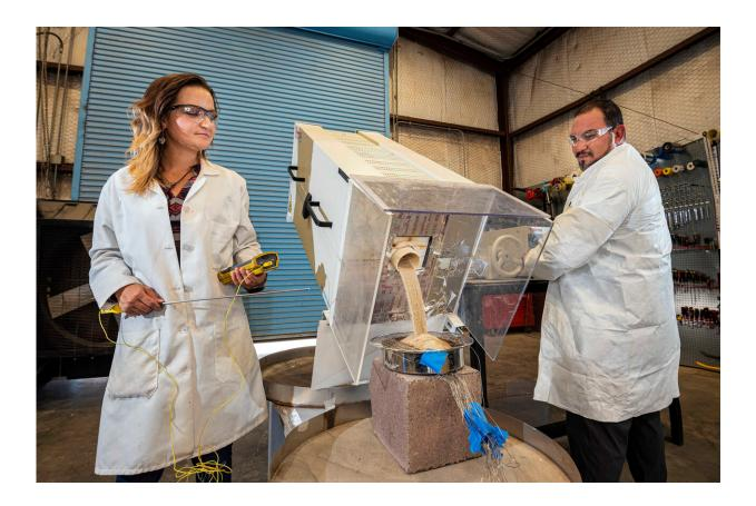
Sandia National Laboratories research team members Jessica Kruichak and William Chavez tested granular calcite and sand against lead oxide. The granular calcite and lead oxide had a leavening and cooling reaction, whereas the sand did not produce a reaction. Credit: Randy Montoya
