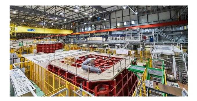
The outer structures (red) for two prototype DUNE detectors that are currently being evaluated at CERN. (Image: CERN)
