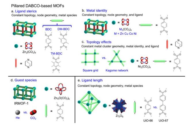
Overview of design strategies for thermal expansion control in nanoporous metalorganic frameworks. a: Modifying the steric bulk of the ligand. b: Changing the identity of the metal in the inorganic cluster. c: Altering the framework topology. d: Varying the guest species. e: Altering the length of the ligand. Credit: HIMS / Advanced Functional Materials
