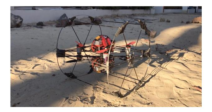
A prototype of the transforming robot Shapeshifter is tested in the robotics yard at NASA's Jet Propulsion Laboratory. Shapeshifter is made of smaller robots that can morph into rolling spheres, flying drones, swimming submersibles, and more. Credit: NASA/JPL-Caltech
