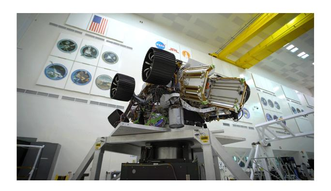
This time-lapse (speeded up 28 times) shows NASA's Mars 2020 rover as it was rotated on a spin table in the clean room of the Spacecraft Assembly Facility at NASA's Jet Propulsion Laboratory in Pasadena, California. Engineers were looking to establish the rover's center of gravity, or the point at which weight is evenly dispersed on all sides. The imagery was taken on Aug. 29, 2019. Credit NASA/JPL-Caltech
