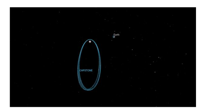
Highly elliptical, a near rectilinear halo orbit around the Moon takes advantage of a precise balance point in the gravities of Earth and the Moon and creates a stability that is ideal for long-term missions like Gateway. Credit: Advanced Space
