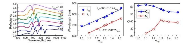
In a less symmetric dielectric environment (that is for smaller nsup), the conventional SLR has a lower quality factor but the novel SLR has a higher quality factor. Credit: SIAT
