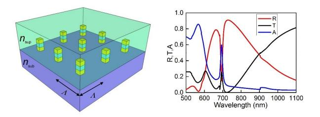
Novel SLR supported by MIM array and its Fano-shaped dip within a broad reflection spectrum. Credit: SIAT
