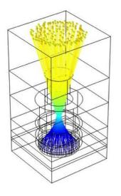
Electron emission trajectory through the vacuum transistor from the source (bottom) to the drain (top). Credit: Jin-Woo Han.
