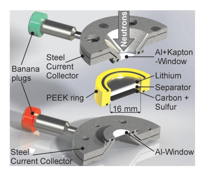
he operando cell was developed at HZB and allows to analyse processes inside the battery during charging cycles with neutrons. Credit: S. Risse/HZB
