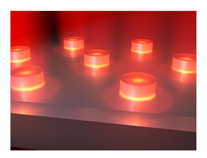
Nanoscale thermal emitters created at Rice University combine several known phenomena into a unique system that turns heat into light. The system is highly configurable to deliver light with specific properties and at the desired wavelength. (Illustration by Chloe Doiron/Rice University) Credit: Chloe Doiron/Rice University
