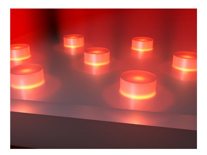
Nanoscale thermal emitters created at Rice University combine several known phenomena into a unique system that turns heat into light. The system is highly configurable to deliver light with specific properties and at the desired wavelength. (Illustration by Chloe Doiron/Rice University) Credit: Chloe Doiron/Rice University
