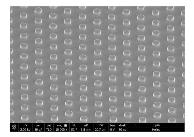
An electron microscope image shows an array of thermal light emitters created by Rice University engineers. The emitters are able to deliver highly configurable thermal light. Credit: The Naik Lab/Rice University
