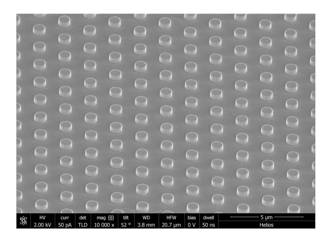
An electron microscope image shows an array of thermal light emitters created by Rice University engineers. The emitters are able to deliver highly configurable thermal light. Credit: The Naik Lab/Rice University
