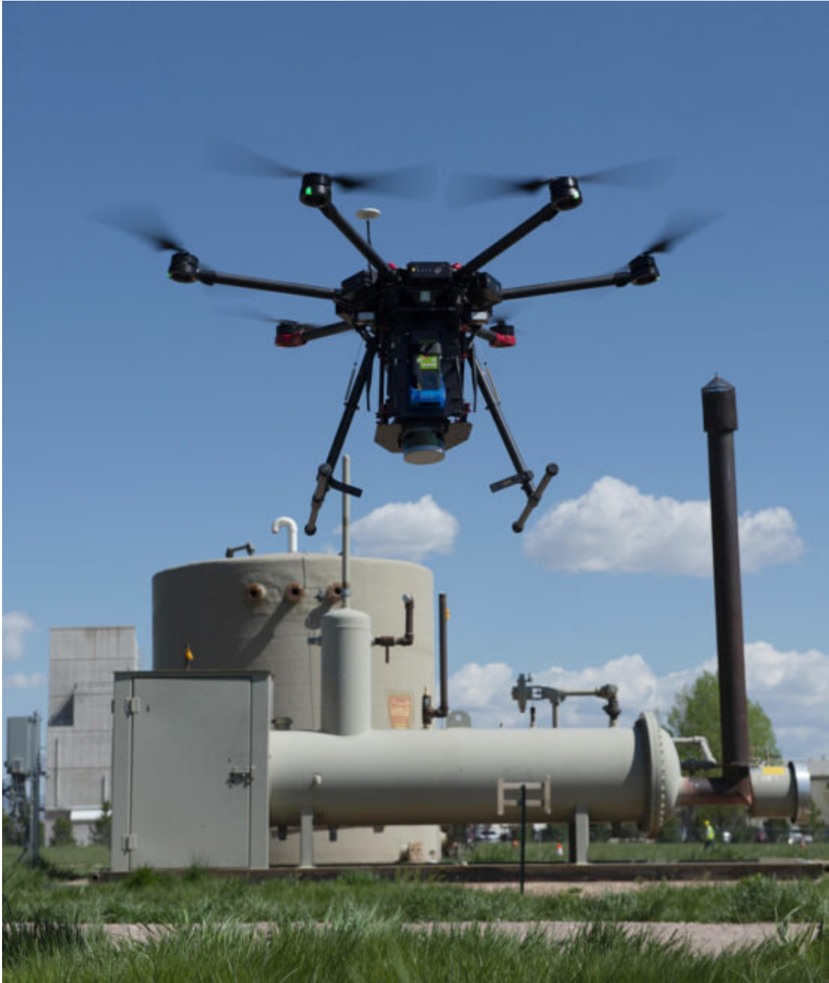
A drone sniffs for methane leaks in the Mobile Monitoring Challenge at the test site in Colorado. Credit: Sean Boggs/Environmental Defense Fund
