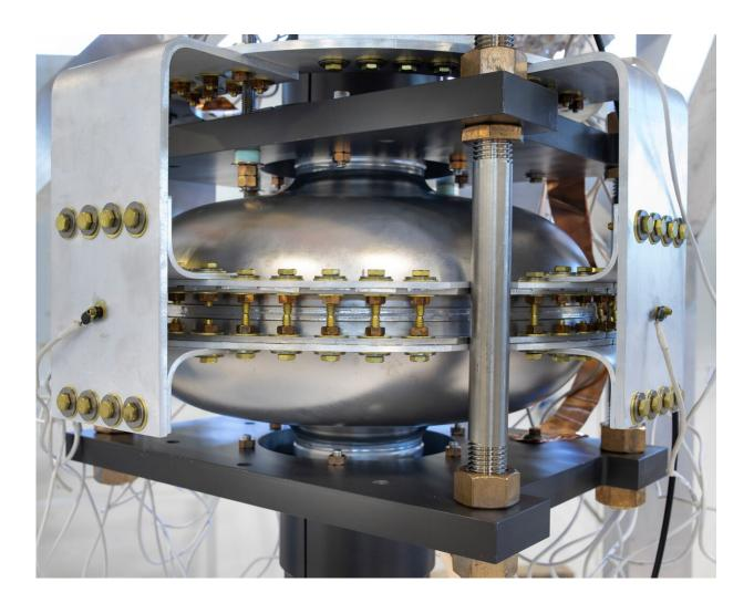
For the first time, a team at Fermilab has cooled and operated a superconducting radio-frequency cavity — a crucial component of superconducting particle accelerators using cryogenic refrigerators, breaking the tradition of cooling cavities by immersing them in a bath of liquid helium. It achieved an accelerating gradient of 6.6 million volts per meter. Credit: Marty Murphy
