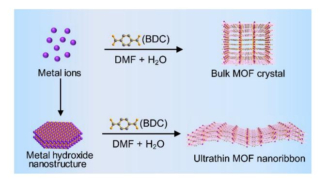
Comparison of the traditional approach for preparation of bulk MOF crystal (top) and metal hydroxide nanostructure precursor approach for synthesis of ultrathin MOF nanoribbon (bottom). Credit: ©Science China Press
