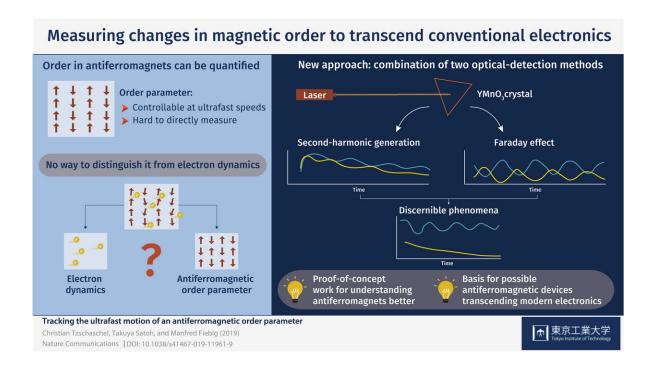
Combination of Faraday rotation and second-harmonic generation obtained the trajectory of an optically induced coherent spin precession. The time-resolved SHG is a valuable tool for the study of antiferromagnetic spin dynamics providing complementary information that is inaccessible by other techniques. Credit: Tokyo Tech
