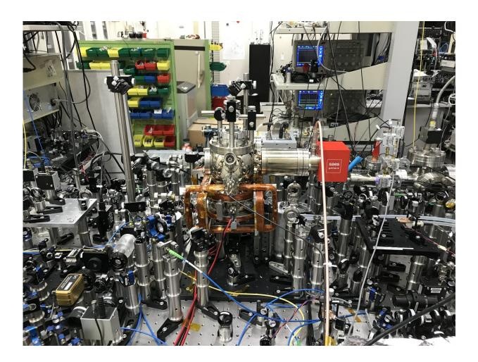
At present the optical lattice clock is a complex arrangement of optical and electronic components. Credit: (c) 2019 Katori et al.
