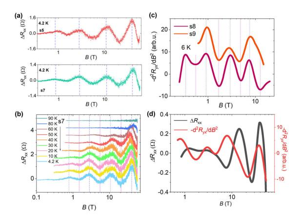
(a) Log-periodic MR oscillations in HfTe5 after subtracting the background. (b) Temperature dependence of the logB-periodic oscillations. (c) Signals of logB-periodic oscillations in the Hall traces of HfTe5. (d) Comparison of the oscillations in MR and Hall traces for the same sample. Credit: ©Science China Press
