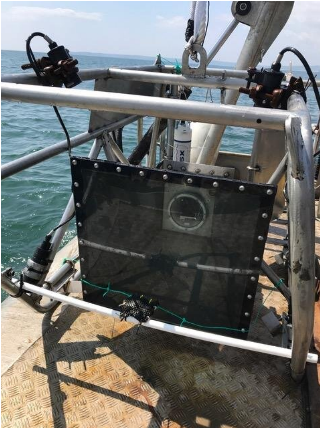
A clear liquid optical chamber (CLOC) fixed to a baited remote underwater video (BRUV) system. Credit: Swansea University
