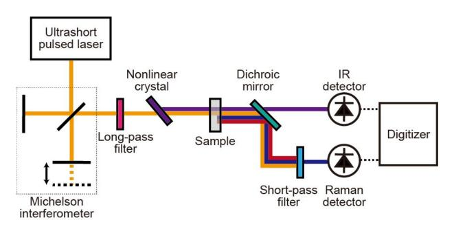
Complementary vibrational spectroscopy is based on a dual-modal Fouriertransform spectrometer with an ultrashort pulsed laser. The Raman measurement is made by Fourier-transform coherent Raman scattering spectroscopy. The infrared measurement is made by Fourier-transform infrared absorption spectroscopy with infrared light generated at a nonlinear crystal. Credit: Takuro Ideguchi
