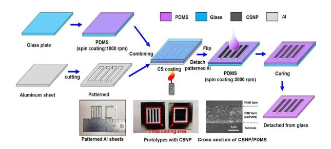
Fabrication process of patterned candle soot (CS) nanoparticle (NP) polydimethylsiloxane (PDMS) patch. Credit: Taeyang Kim
