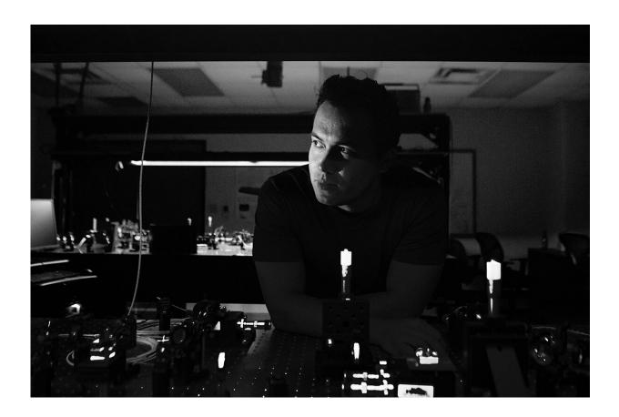
Omar Magaña-Loaiza observes his efficient source of spontaneous parametric down-conversion. This source uses a nonlinear crystal to produce correlated photon pairs. Credit: Elsa Hahne, LSU
