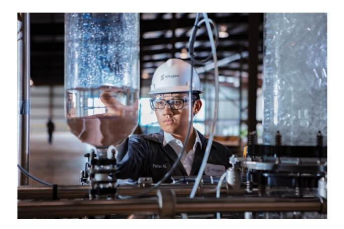
Solugen's proprietary process for producing hydrogen peroxide uses modified enzymes and inexpensive compounds like sugar. It is currently being used in two pilot facilities that create more than 10 tons of the chemical every day. Credit: Solugen
