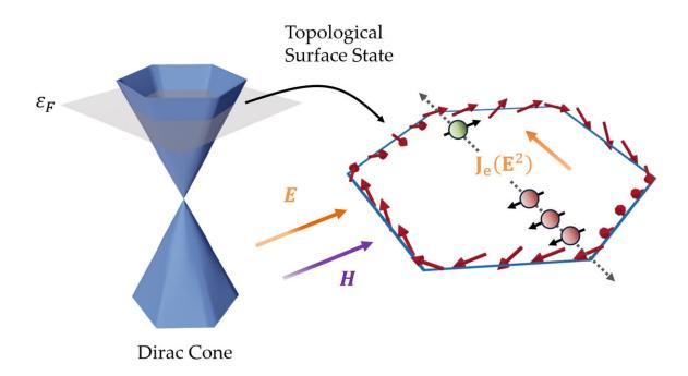
The specific relation between electronic states in a topological insulator and momentum leads to an asymmetric accumulation of spin, depicted on the right, which gives rise to an electric current to second order in an applied electric field E. Credit: Shulei Zhang / Argonne National Laboratory
