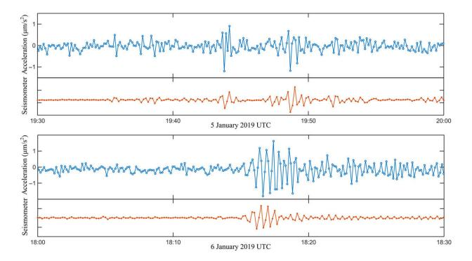
Earthquake seismic waves detected in Berkeley. The atomic gravimeter measures the vertical acceleration of the seismic waves with an update rate of 0.13 Hz. The seismic signal is the vertical channel of the seismometer located in Haviland Hall in the University of California (UC) Berkeley campus. It is in arbitrary unit and has an update rate of 0.1 Hz. Credit: Science Advances, doi: 10.1126/sciadv.aax0800.
