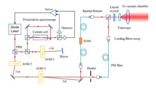
Schematic of the laser system. AOM, acousto-optic modulator; EOM, fiber-based electro-optic modulator; PBS, polarization beam splitter; PM fiber, polarization maintaining fiber. Credit: Science Advances, doi: 10.1126/sciadv.aax0800
