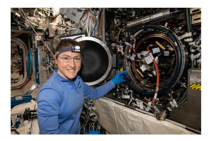
NASA astronaut and Expedition 59 Flight Engineer Christina Koch works inside the US Destiny laboratory module's Combustion Integrated Rack. She was replacing hardware for a series of experiments collectively known as Advanced Combustion via Microgravity Experiments (ACME). Credit: NASA
