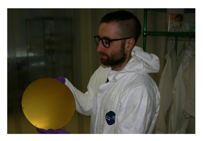
Yassid Ayyad, detector systems physicist at the National Superconducting Cyclotron Laboratory at Michigan State University, is part of the research team that observed a rare decay in the exotic beryllium-11 nucleus. Here he holds the pad plane of the Active Target Time Projection Chamber detector that was used in the experiment. Credit: National Superconducting Cyclotron Laboratory
