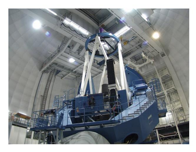
3.5-m telescope at the Calar Alto observatory where the CARMENES spectrograph is installed. Credit: Pedro Amado/Marco Azzaro - IAA/CSIC
