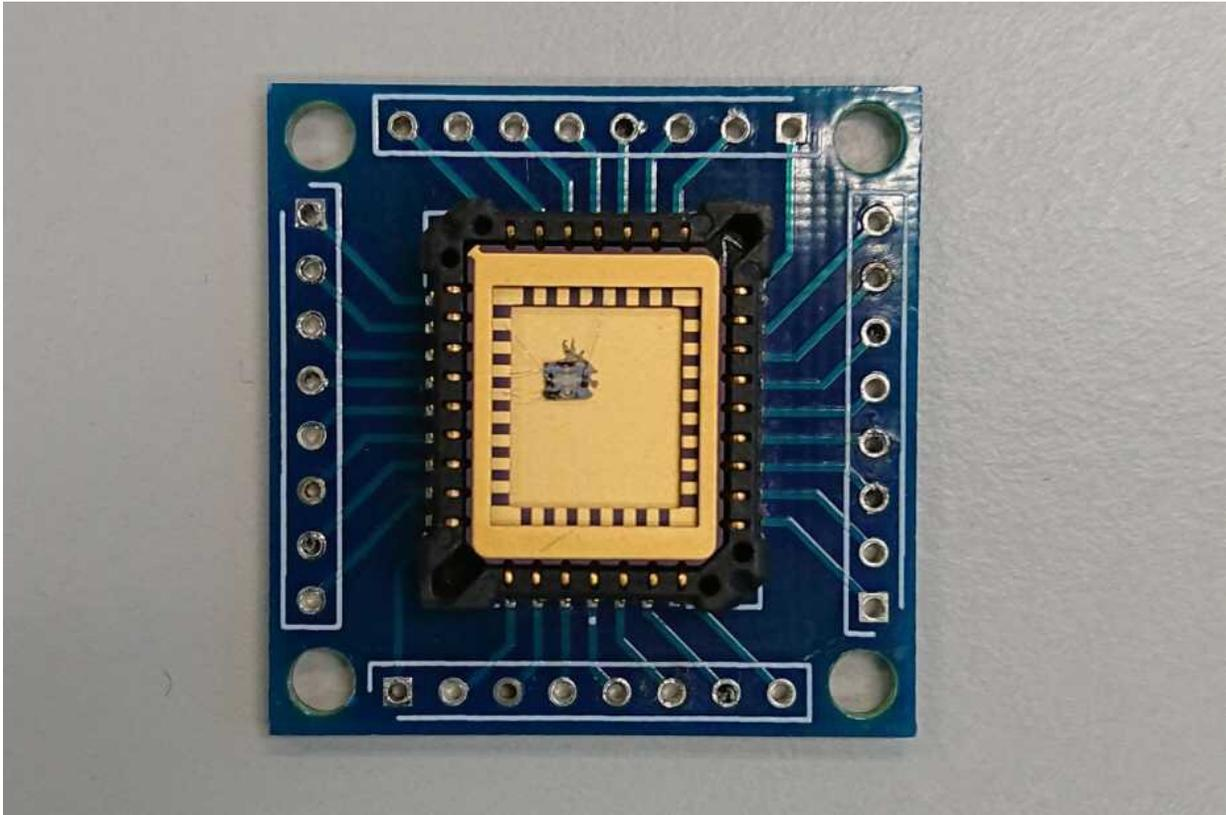
The millimetre-sized black dot in the centre of the gold section is the alcohol sensor. Credit: ETH Zurich
