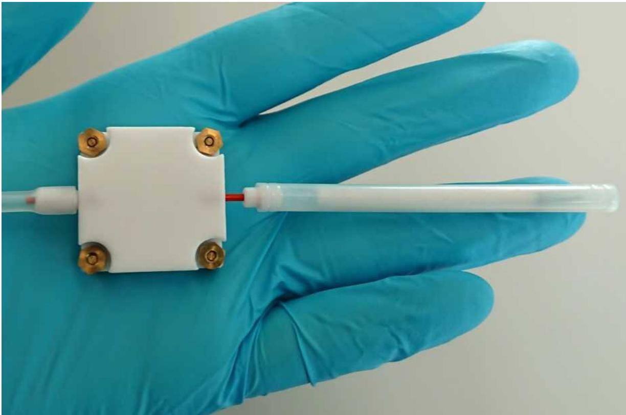
In this image, the sensor is inside the white casing. To its right is the polymer tube in which methanol is separated from ethanol. Credit: Van den Broek J et al. Nature Communications 2019
