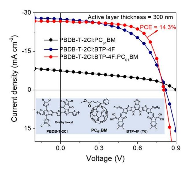
The J-V characteristics for OSCs based on PBDB-T-2Cl: BTP-4F, PBDB-T-2Cl: PC61BM and PBDB-T-2Cl: BTP-4F: PC61BM; the chemical structures of
