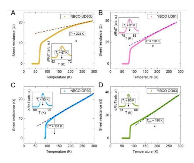
Sheet resistances of the NBCO and YBCO films as a function of the temperature. The sheet resistance  $R\Omega$  is plotted as a function of the temperature for (A) sample UD60b (thickness: 100 nm; deposited in the same conditions as
