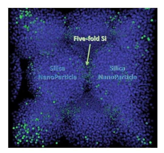
Plasticity-carriers (five-fold silicon shown here) form at the contact of silica nanoparticles under extreme pressure, in route to a fully dense ductile silica glass Credit: Rensselaer Polytechnic Institute
