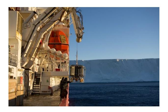
CTD (Conductivity, Temperature, Depth) instrument being lowered into the ocean from the RRS James Clark Ross. Credit: British Antarctic Survey
