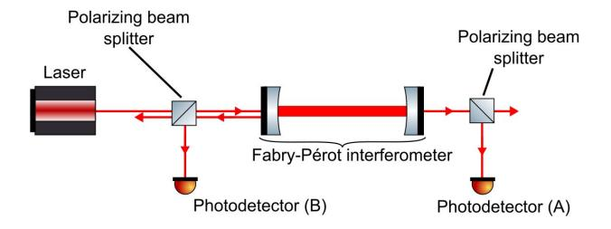
A schematic for the proposed instrument to hunt for axion dark matter. The project is ongoing at the University of Tokyo Institute for Cosmic Ray Research. Credit: 2019 Nagano et al
