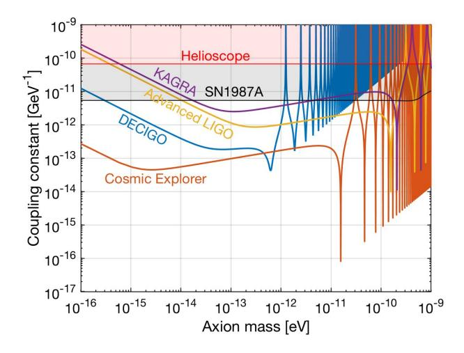
This chart compares the sensitivity of gravitational-wave detectors suitable for the axion hunt. The project is ongoing at the University of Tokyo Institute for Cosmic Ray Research. Credit: Nagano et al
