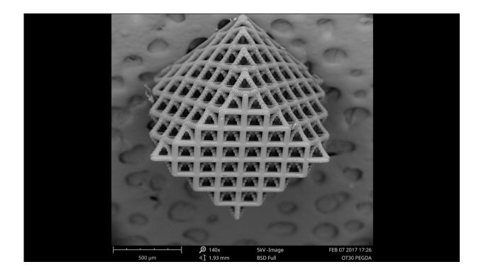
Scanning electron microscopy images of a classic octet lattice and topologically optimized, isotropic oblate and quasi-spherical octahedral lattice built with a projection micro-stereolithography 3-D-printing technique. Credit: Lawrence Livermore National Laboratory
