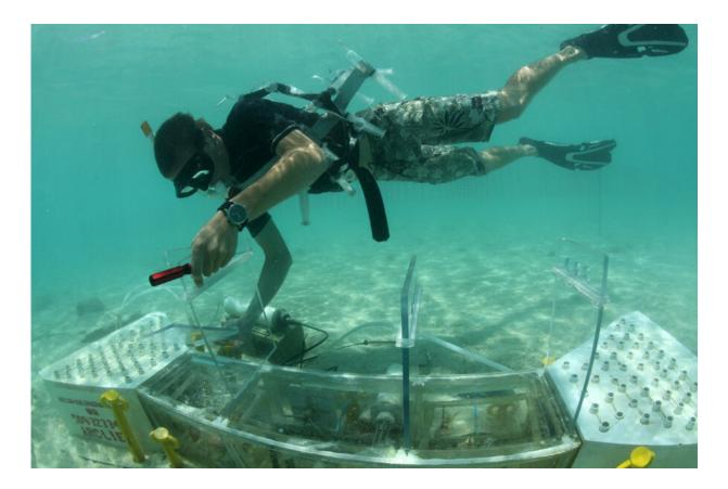
A member of the team snorkeling at low tide to sample the seawater in each chamber (there is a carabiner of sampling syringes around his arm) and to temporarily insert guillotine style doors in order to seal the chamber for 2 hours in order to measure the corals rates of calcification/dissolution and photosynthesis/respiration. Credit: David Kline
