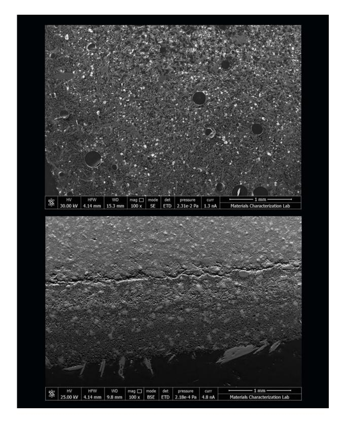
These images compare cement pastes mixed in space (above) and on the ground (below). The sample from space shows more porosity, or open spaces in the
