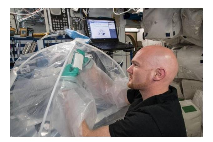
European Space Agency astronaut Alexander Gerst works on the MICS experiment aboard the International Space Station. Observations of how cement reacts in space during the hardening process may help engineers better understand its microstructure and material properties, which could improve cement processing techniques on Earth and lead to the design of safe, lightweight space habitats. Credit: NASA
