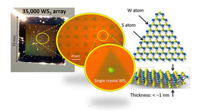
A substrate (left photograph) that is fabricated by integrating about 35,000 monolayer single crystals of WS2, and a structural schematic of the monolayer single crystal of WS2 (right figure). Credit: Toshiaki Kato
