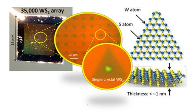
A substrate (left photograph) that is fabricated by integrating about 35,000 monolayer single crystals of WS2, and a structural schematic of the monolayer single crystal of WS2 (right figure). Credit: Toshiaki Kato
