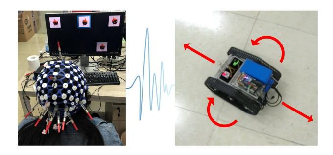
A cap containing a new type of EEG electrode can be used to control a toy car with brain waves. Credit: Adapted from *Nano Letters* 2019, DOI: 10.1021/acs.nanolett.9b02019
