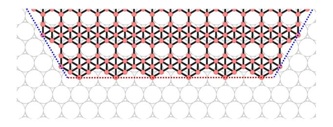
An illustration shows how edges are connected at the corners of a borophene flake. Materials scientists led by Rice University have predicted that the shape of borophene, the 2D allotrope of boron, can be controlled. Credit: Zhuhua Zhang/Rice University/Nanjing University of Aeronautics and Astronautics
