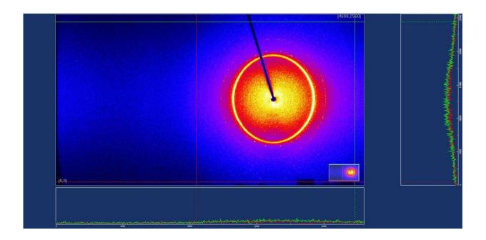
A sample from the study undergoing X-ray diffraction. The chemical makeup of the sample is determined by interpreting the distinct deflection patterns of the X-rays. Credit: Nick Crouch
