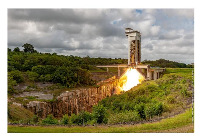
On 28 January 2019, the first qualification model of the P120C solid-propellant motor, in the configuration for Vega-C, was static fired on the test stand at Europe's Spaceport in French Guiana. Credit: European Space Agency
