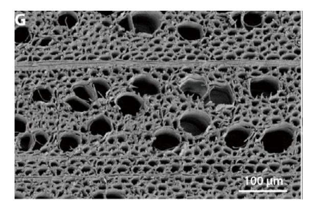
Cross section of nano wood membrane used for water filtration. Credit: D. Hou, University of Colorado.
