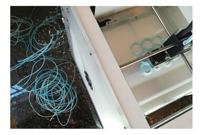
Ocean plastic, turned into filament for use in a 3-D printer. Credit: Ian Lambert, Author provided
