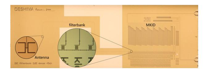
Radio signals collected by the telescope are injected into the on-chip antenna (on the left) and propagate to the right-hand side through the thin metal line. A filterbank is located along the line and signals with specific frequencies are extracted by each filter. The signal then enters the MKID and is detected. The size of the chip is 4 cm x 1.5 cm. Credit: Delft University of Technology
