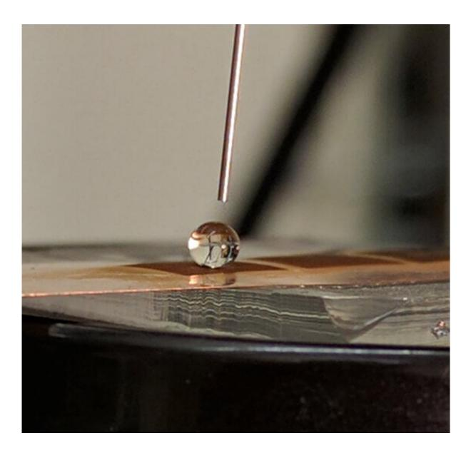
This image shows a water drop on a created superhydrophobic surface, showing a very high contact angle. Purdue University researchers developed a new
