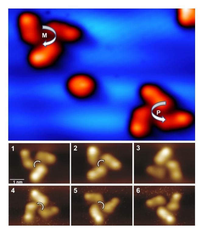
A look at how the propeller is made up and the unidirectional rotations. Credit: Saw-Wai Hla
