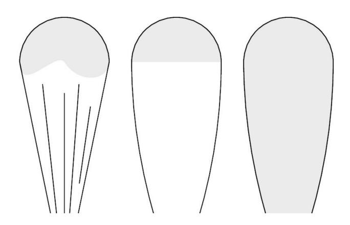
Steam balloon variants. During ascent the ambient pressure decreases and consequently the gases expand. If the balloon is filled by steam partially (Variant 1), the expanding steam eventually fills the balloon. If the lower part is filled by hot air (Variant 2), extra air flows out from the bottom during the ascent. If the balloon is filled by steam entirely (Variant 3), the exiting gas is steam. Credit: Finnish Meteorological Institute
