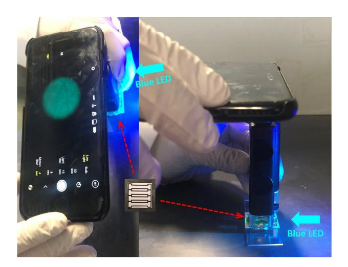
A sensitive new device can detect tiny amounts of norovirus in water. Credit: American Chemical Society
